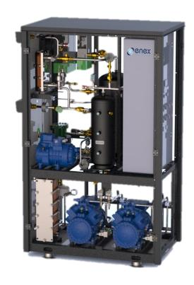
Enex presents TAGO, the new range of transcritical  $CO_2$  refrigeration units, designed to combine compactness and high reliability. Available in 7 sizes with 2 MT compressor and 1 LT compressor, it is only 800 mm wide. With its tower shape, it is ideal for installation in plant rooms with restricted footprint and/or where access is through narrow doors.
