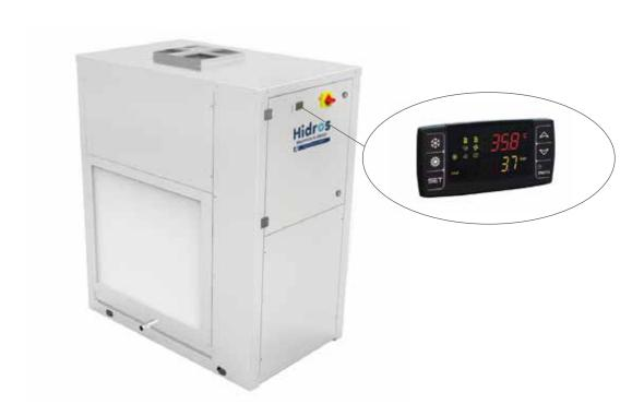
Series SMA dehumidifier are expressly designed for use in swimming pools where humidity should be closely controlled in order to guarantee optimal comfort. These units are intended to be installed in a technical room close to the swimming pool. A centrifugal fan with high available static pressure allows unit connection to ductworks, both for air suction and discharge. This series comprises 6 basic models which cover a capacity range from 263 to 940 l/24h.
